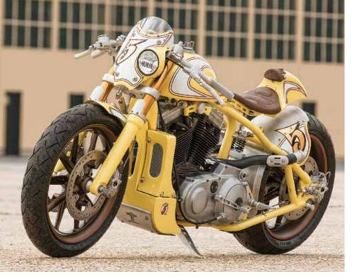
is aluminum, with two sheet metal panels inspired by motocross racers, and Steve hammered that centerpiece on a tree stump before rolling it into shape. Necessity is the mother of all invention.
